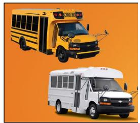
**B**: Vehicle type B has been retired and not selectable. Previously reported vehicles will remain as vehicle type B. This was constructed utilizing a stripped van or truck chassis with the entrance door behind the front wheels.
